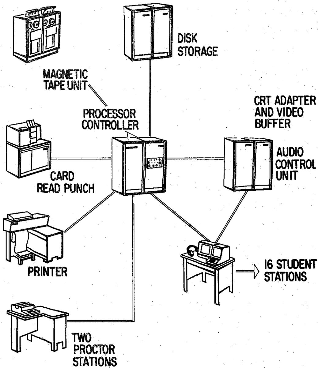
Figure 1. System configuration for Stanford CAI System.
